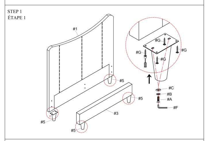
Do not tighten screws until completely assembled./
