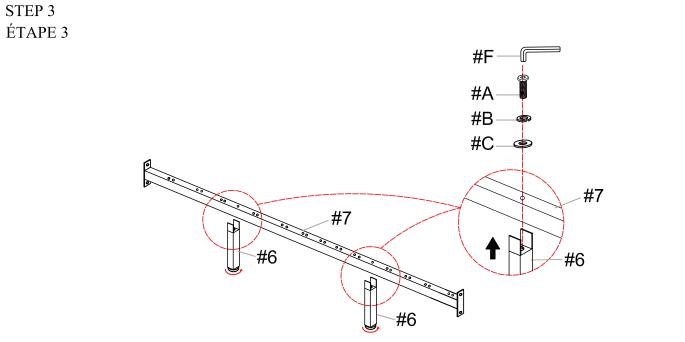
Do not tighten screws until completely assembled./
