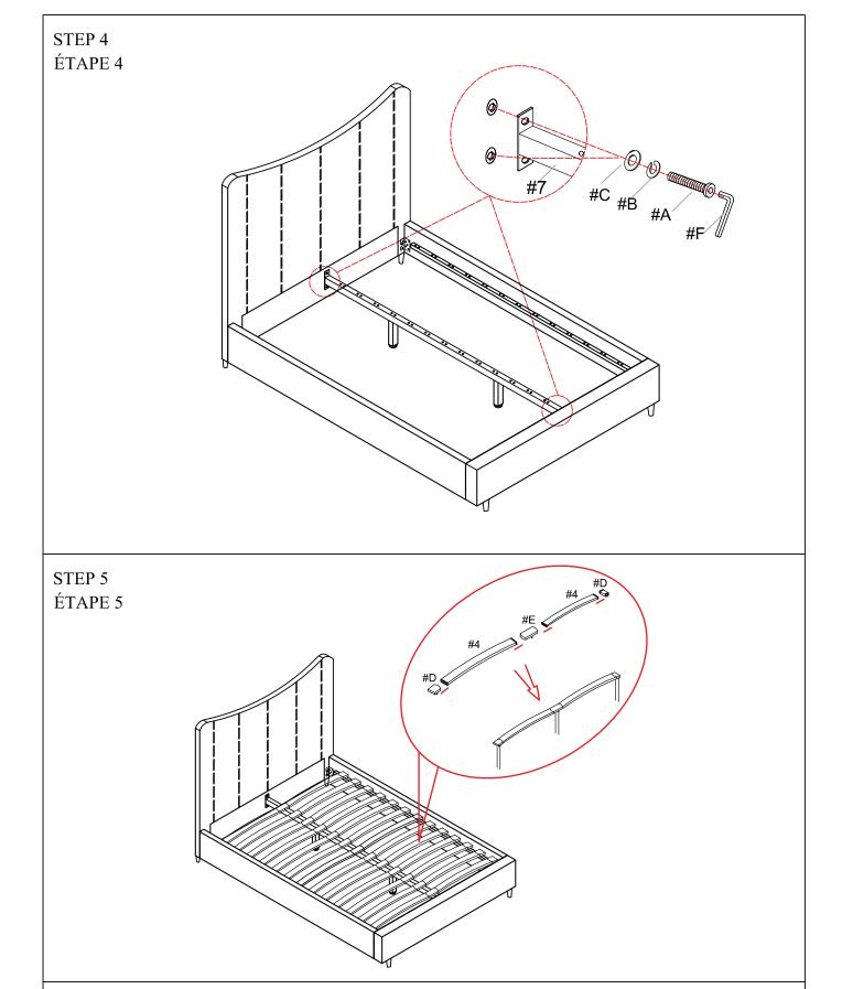
Do not tighten screws until completely assembled./
