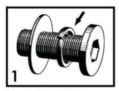
Before attaching each of the screws, make sure that the **smaller lock washer is between** the larger washer and the head of the screw.
