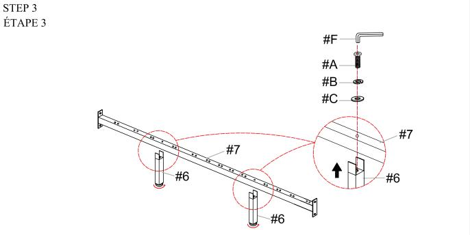
Do not tighten screws until completely assembled./
