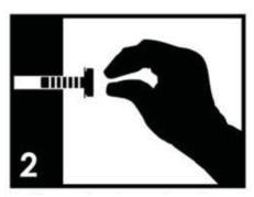
Position each part correctly and insert all screws into their respective holes. Then, **hand-tighten** only until 70% tight. Complete tightening with the tools will come at a later step.
