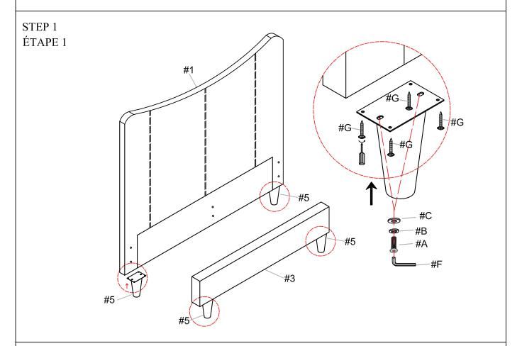
Do not tighten screws until completely assembled./
