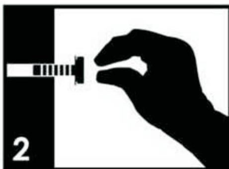
2 Position each part correctly and insert all screws into their respective holes. Then, **hand-tighten** only until 70% tight. Complete tightening with the tools will come at a later step.
