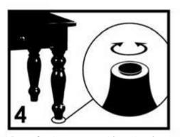
Some furniture come with optional **height adjustment knobs** underneath each leg. Turn this knob counterclockwise to raise the leg level or clockwise to lower the leg level.
